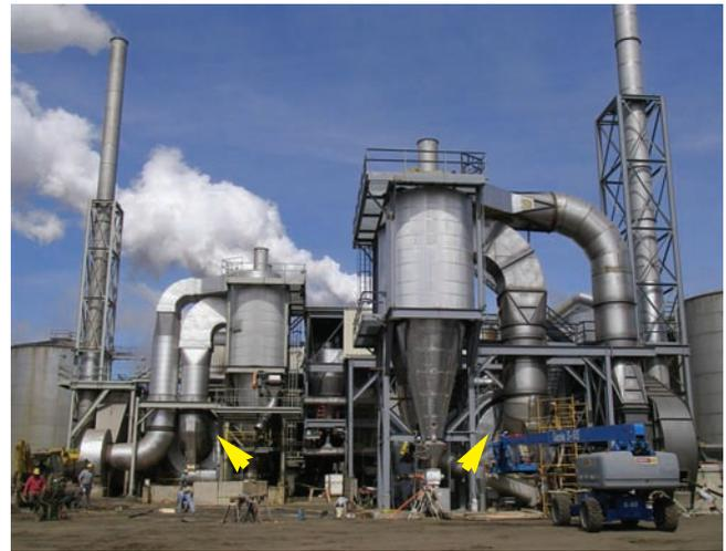
**Two rotary drum steam-atmosphere dryers (arrows) process distillers spent grain in an ethanol plant. Heat energy from their exhaust is used in evaporators and the noncondensable vapor is recirculated to the furnace to reduce the dryers' fuel consumption.**
