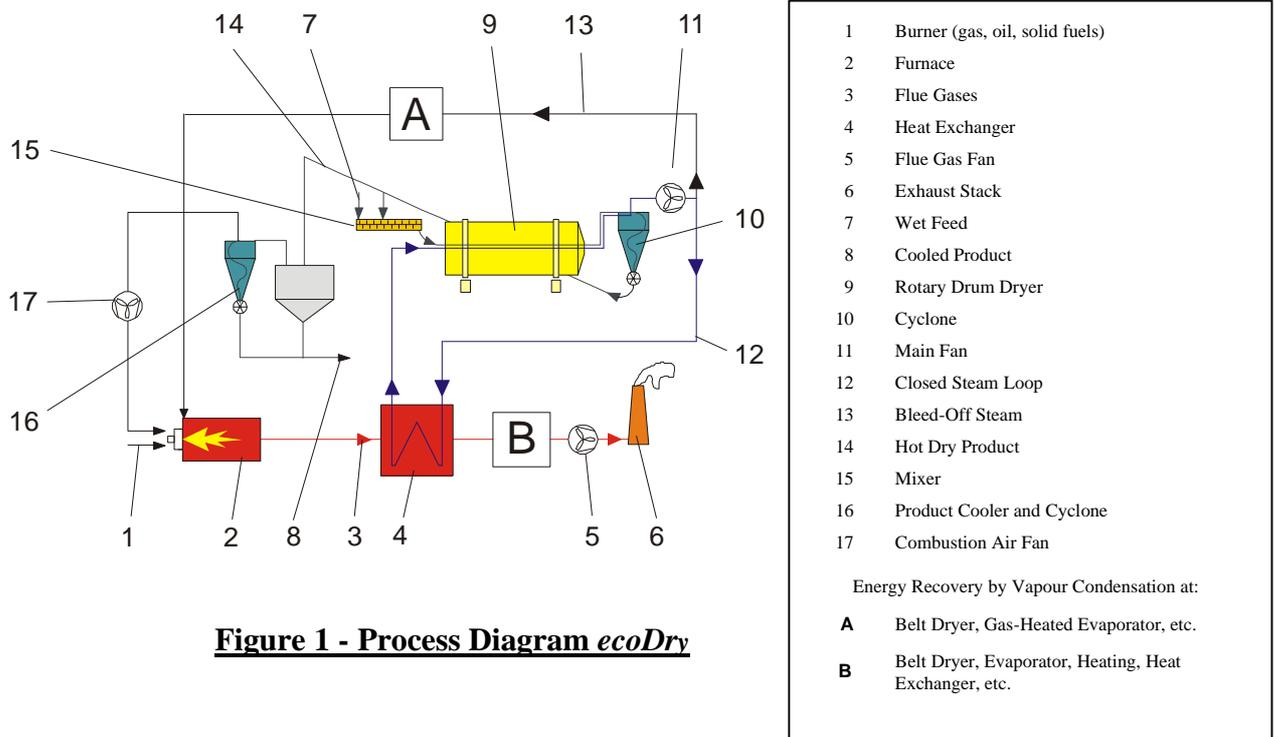
**Figure 1 - Process Diagram *ecoDry***
