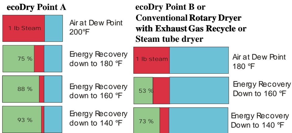
**Figure 4 - Energy Recovery through Vapor Condensation**
