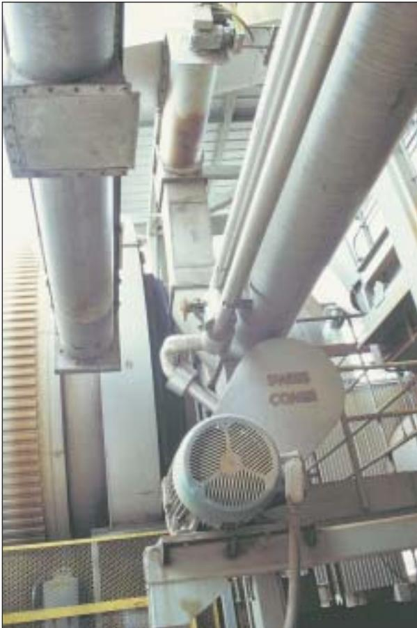
Pipelines and chute (upper right) deliver centrifuged solids, evaporated syrup and dry finished product to Swiss Combi mixer.
