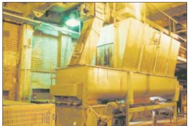
Centrifuged solids drop into ecoDry dosing bin, mounted on weight sensors to automatically optimize flow into mixer and dryer.
