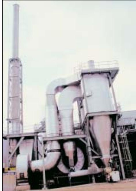
*Swiss Combi dryer "back end": DDGS emerges from rotating drum onto tightly enclosed conveyor while ducts take process steam up to cyclones and back to the heat exchanger intake. Stack framed against blue sky attests to exhaust clarity.*
