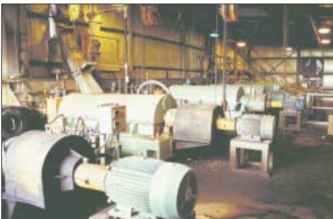
Centrifuges receive whole stillage and separate grain solids from "thin stillage".
