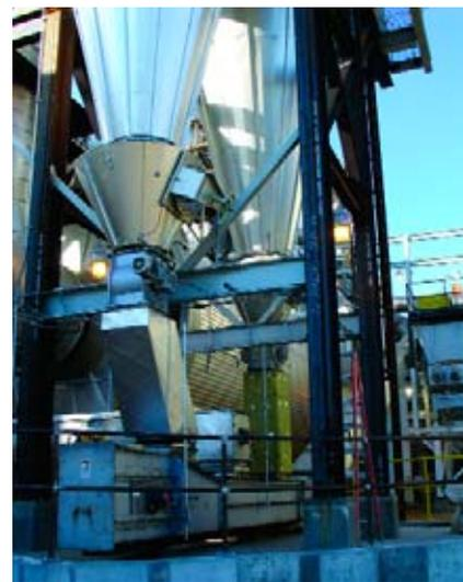
***These cyclones remove entrained particles from the steam exhausted by the rotary drum dryer, dropping the particles into the tightly sealed mechanical conveyor (below cyclones) for transfer with the finished DDGS to a cooler.***
