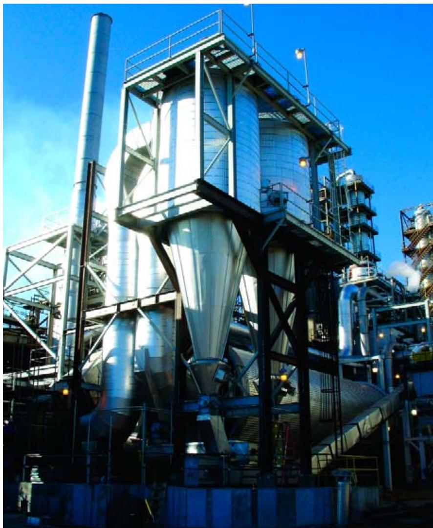
*The new closed-steam-loop drying system consumes its own pollutants, producing clear exhaust (at left) that contrasts sharply with the haze exhausted by the old system. The new rotary drum dryer, with the large steam exhaust duct exiting from it, is at the lower right.*
