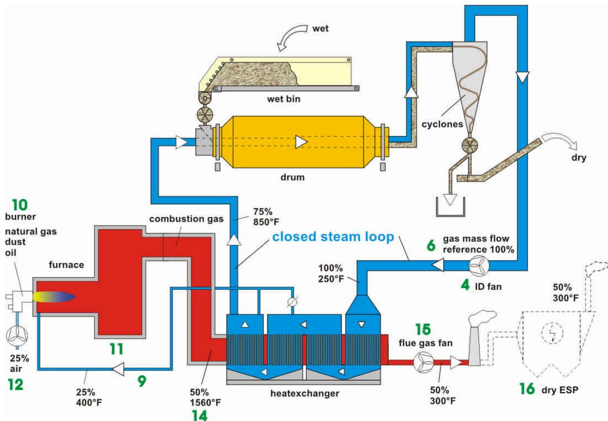
The diagram shows a typical arrangement of a natural gas, sanding dust or oil burner (10) with furnace (11). The figure shows that the bled off steam, which we call "inert gas"(9), is directed to the front end of the primary combustion chamber. This "inert gas" is there mixed with the flame for oxidation of the VOC's, carbon monoxide etc. To assure maximum destruction or oxidation, a temperature of about 1560 °F (1500 - 1600 °F) (14) is needed.
