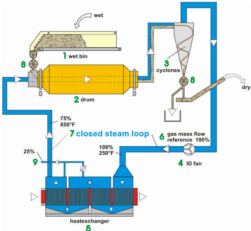
The wet strands or wood particles are fed in the known manner from the wet bin (1) into the drum (2). Dry, they are separated after the drum from the drying gas in a drop out chamber and/or cyclones, here shown only as one cyclone (3).
