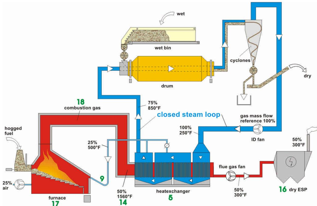
This figure shows a wet fuel heating furnace (17) including how the inert gas (9) can be introduced to an inclined grate furnace system without disturbing the combustion. Depending on type of furnace, part of the inert gas can be added through the normal secondary gas nozzles (not shown). The arrangement of the ducting between furnace and heat exchanger must be realized assuring good mixing of the flue gas for VOC destruction and burn out of sparks.
